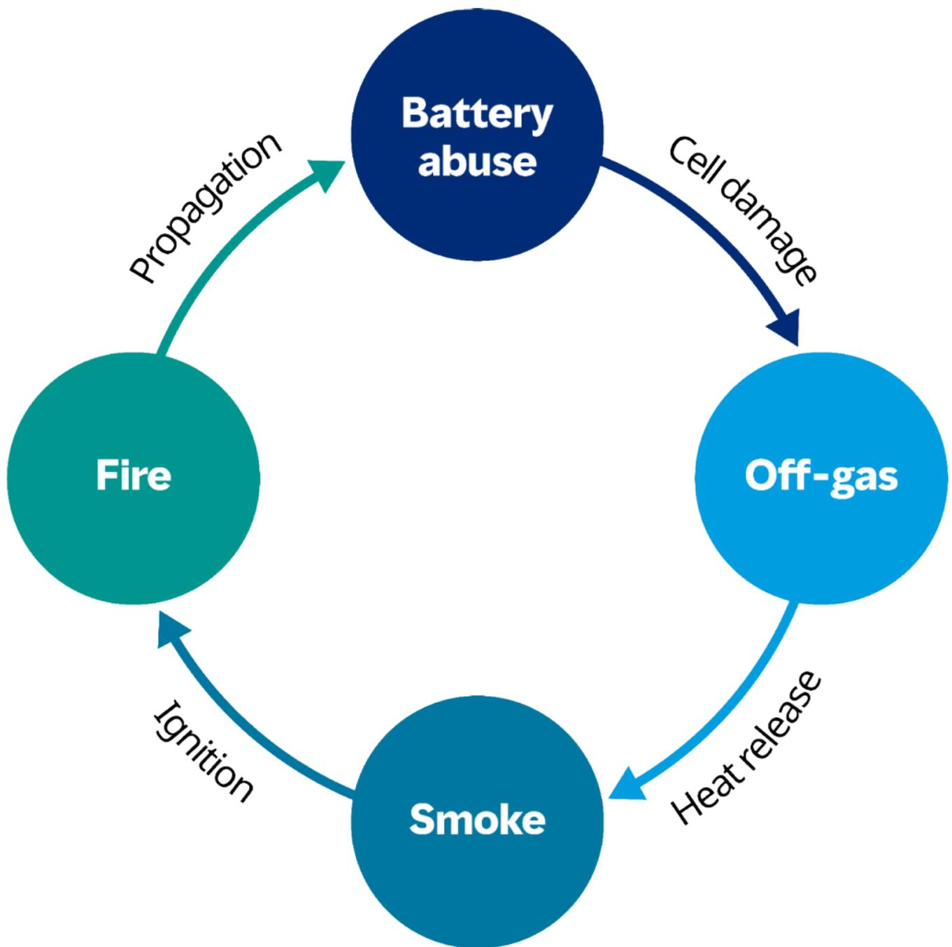
**Figure 1:** Thermal runaway feedback loop.
